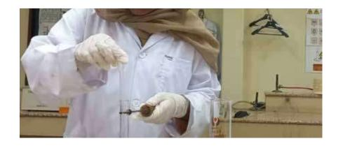
Acidify the water sample: Add a small amount of nitric acid to the water sample to acidify it. This helps to dissolve any metals that may be present in the water and prevents them from precipitating out of solution.
